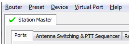
When the USB driver is installed correctly and Station Master is turned on Router will show a device tab with a **GREEN** ✓ beside the device name.
