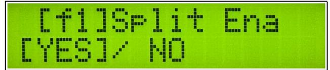
**[f1] Split Ena:** Enable/Disable split TX/RX antenna switching. The split enable status is stored separately for each band.
