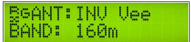
**GRP:** or **G** centered vertically on the LCD indicates that an antenna group or antenna from a group is used.
