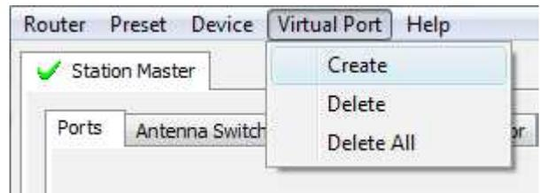
**Create** - Creates virtual COM ports. It is possible to select more ports at once by holding the *Control* key on the keyboard and clicking on COM port numbers. Creating a virtual port may take a while, be patient.
