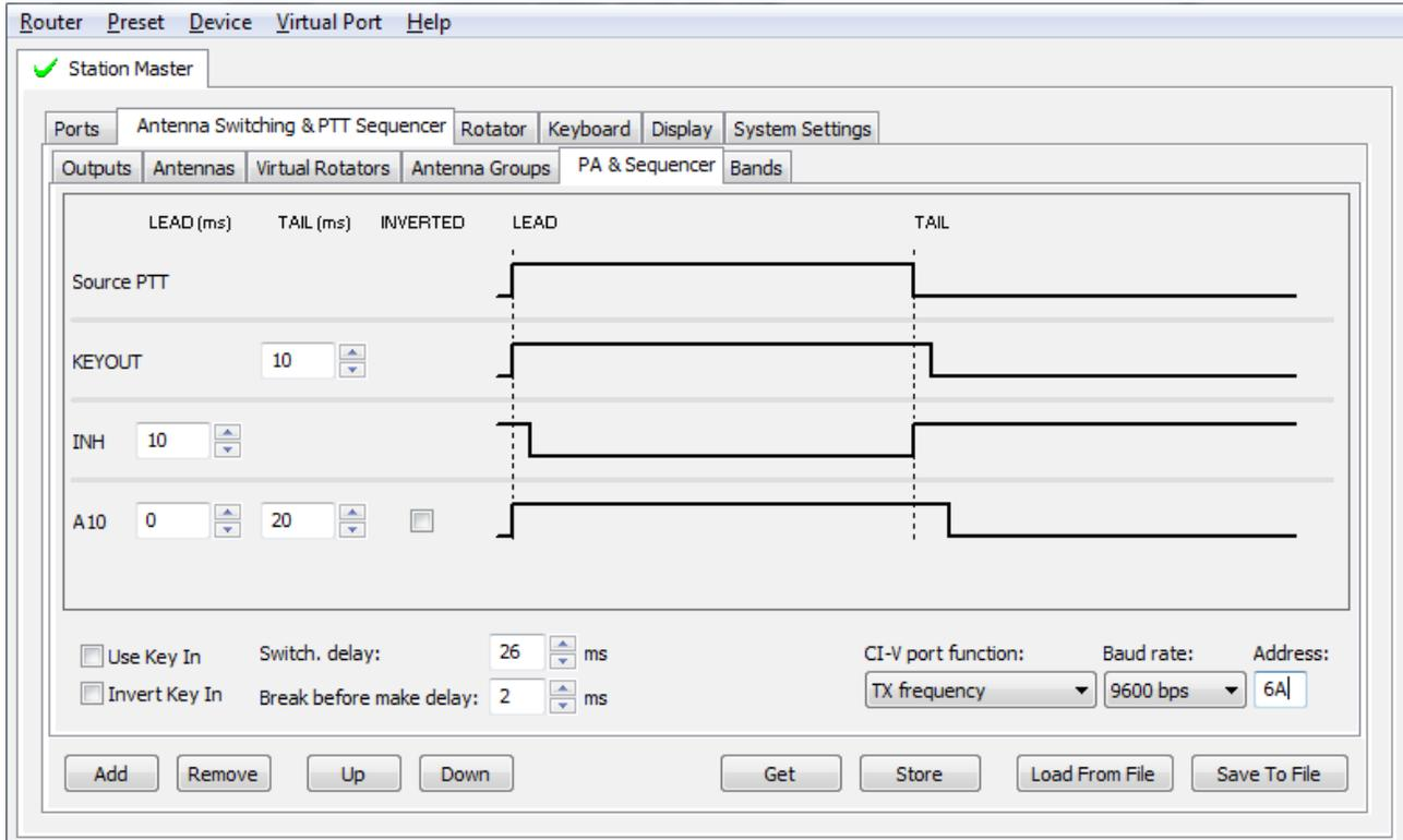
If you are using a power amplifier, it is necessary to control it from the Station Master PA port and not directly from the transceiver. Pin assignments for the signals at the PA connector are in Appendix A. The Power Amplifier port contains several signals:
