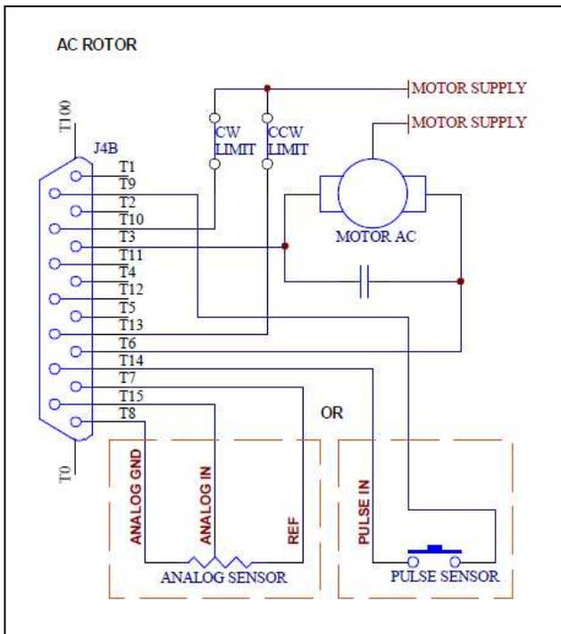
Typical connection for an AC motor
