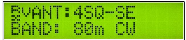
**VR:** or **V** centered vertically on the LCD indicates that a virtual rotator or an antenna from the virtual rotator is being used.
