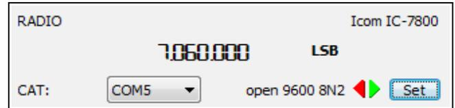
Data flowing through the Control channel is indicated by two arrows. A green arrow shows data flow from the host application to the radio and a red arrow shows data flow from the radio to the application.
