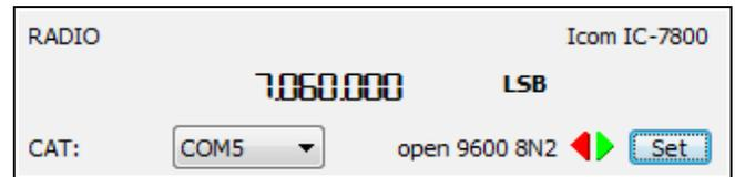
Data flowing through the Control channel is indicated by two arrows. A green arrow shows data flow from the host application to the radio and a red arrow shows data flow from the radio to the application.
