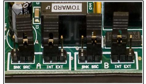
**PORT B:** Contains six (6) outputs with single common terminal (B1-B6) and four (4) outputs (B7B10) with isolated contacts. The common terminal of relays B1-B6 can be configured for internal or external power and source/sink operation by using the PORT B jumpers in the same manner as the PORT A jumpers.
