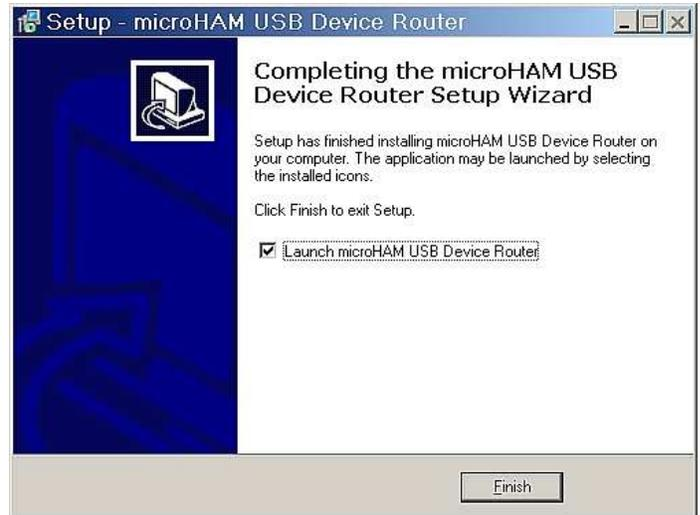
**Plug in the USB cable, turn ON Station Master and proceed to configuring Router for your station and software.**
