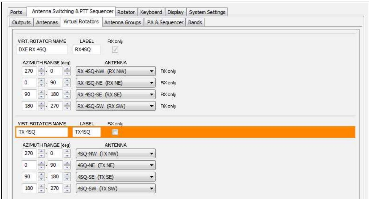
The number of virtual rotators is not limited; a new Virtual Rotator (VR) can be added by **Add** button or a virtual rotor can be deleted by selecting it (orange background) and clicking the **Remove** button.
