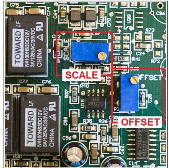
12. The span of the rotator has now been calibrated. To calibrate the absolute azimuth, it is necessary to enter two points as far apart as possible but at least 30 degrees from the limits on each end of the rotation.
