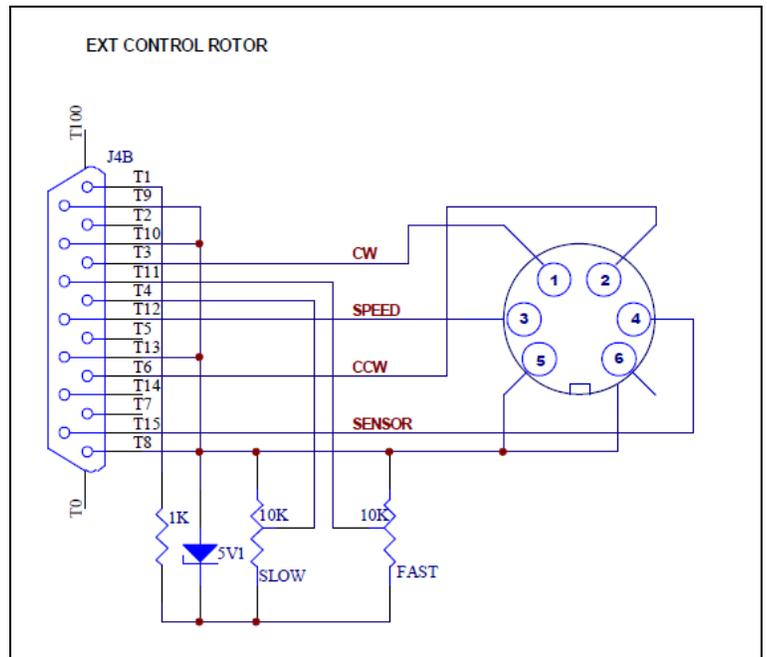
Connection to Yaesu DXA/DXC rotator series.
