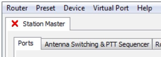
When Router shows a **RED** "X" instead of a green ✓, it means the device is disconnected and Router does not see the USB part of Station Master. This happens when the USB cable is unplugged or the USB driver is not correctly installed.
