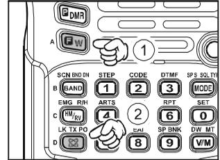
2. Press the **[F/W]** key, followed by the **[∞(LK)TXPO]** key (repeatedly, if necessary) to make the “HIGH” notation appear and restore High Power operation.
