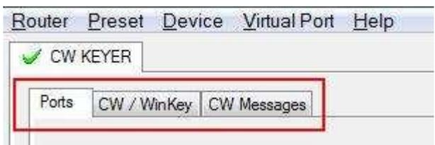
Router must be used to configure CW Keyer for proper operation. The device configuration tab (in the red rectangle) is used to setup each part of the CW Keyer – virtual ports for communicating with the application (Ports), WinKey keyboard CW (keying), and stored CW messages (CW Messages).
