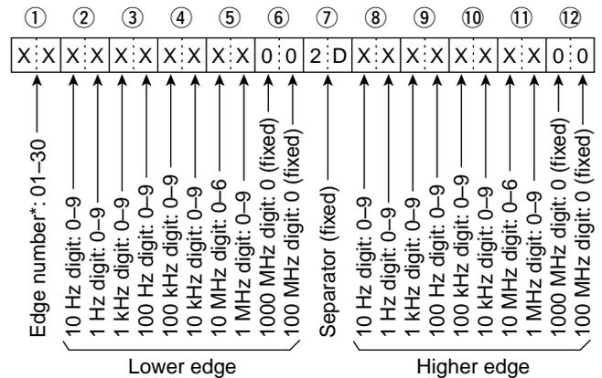
\*Edge number setting is not necessary with command 02.
