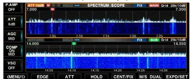
**NOTE:** If a strong signal is received, a ghost waveform may appear. If it appears, push [ATT](F) several times to enable the Scope attenuator.
