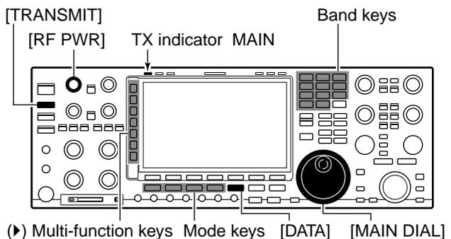
**NOTE:** When the SSB data mode is selected, the audio input from [ACC 1] is used for modulation input instead of [MIC].
