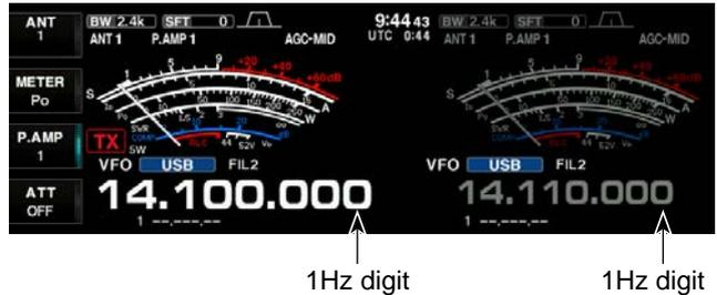
/// **NOTE:** 1 Hz tuning step functions for both Main and Sub bands simultaneously. Therefore, either [TS] can be used to select the 1 Hz tuning steps.
