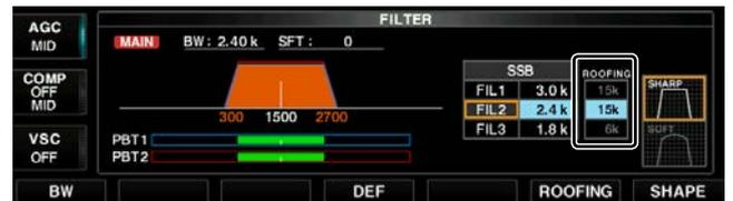
• Roofing filter default value (kHz)
