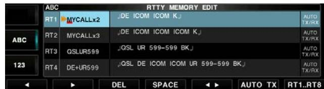
**NOTE:** When no keyboard is connected, the transceiver always functions using the “AUTO TX/RX” setting.
