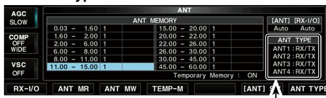
All antennas, connected to [ANT1]~[ANT4], are set as for ‘TX/RX.’
