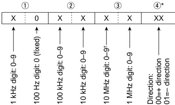
\*No need to enter for transverter offset frequency setting.
