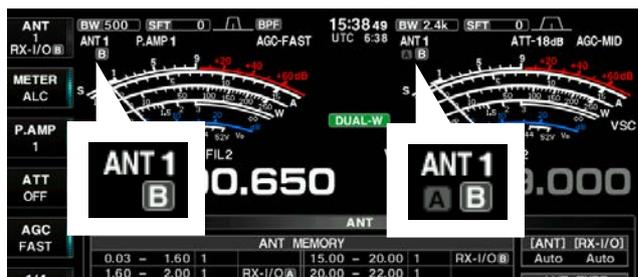
When a common antenna is selected on the Main and Sub bands, different RX-I/O settings cannot be set. Thus, the transceiver automatically sets the RX-I/O setting of the inoperating band to the correct setting, the same as the operating band.
