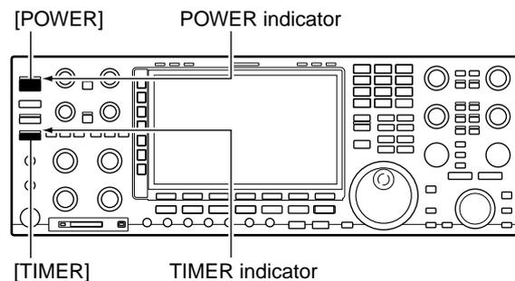
/// The Daily timer action in the Timer set screen must be set to ON to enable the timer operation, described in page 14-5 steps ③.
