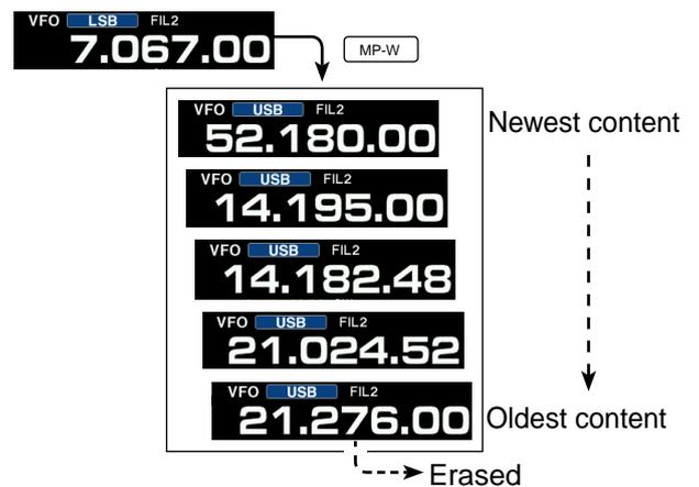
In this example, 21.276 MHz (USB) will be erased when 7.067 MHz (LSB) is entered.
