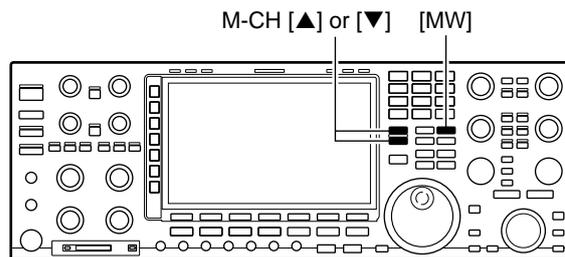
[EXAMPLE]: Programming 7.088 MHz/LSB into memory channel 12.
