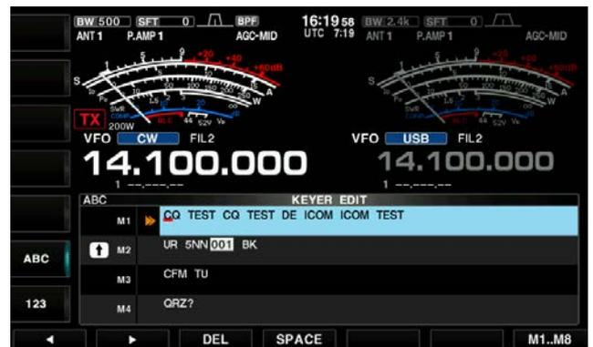
• **Example: Entering “QSL TU DE JA3YUA TEST” into the Memory keyer M3**
