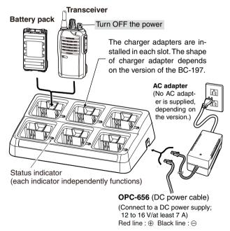
There are two types of BC-197 chargers for the transceier; one is for Ni-MH batteries, and the other is for Li-ion batteries.
