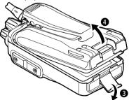
**Be careful!** The latch is tightly locked, so use caution when releasing it. **DO NOT** use your finger nail. Use the edge of a coin or screwdriver tip to carefully release it.
