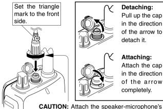
connector securely to prevent accidental dropping, or water intrusion in the connector.
