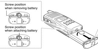
**NOTE:** When removing or attaching the battery pack, use a coin or flat-blade screwdriver to loosen or tighten the bottom screw.
