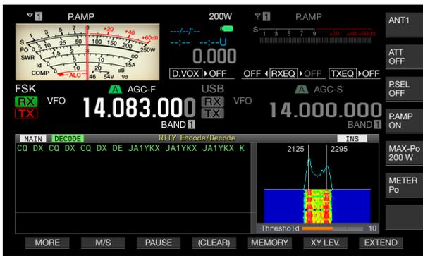
Fig. 89 Example of a RTTY Decode View
