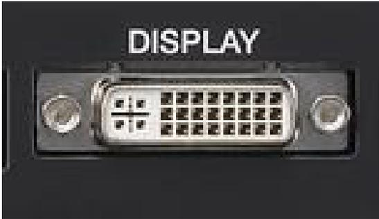
Fig. 139 DISPLAY Connector (on the Rear Panel)
