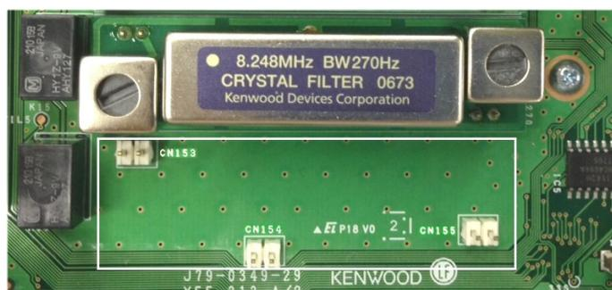
Fig. 16 Additional Roofing Filter Mounting Slot
