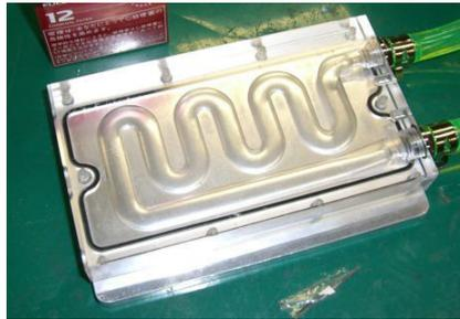
Fig. 5 Water-Cooling Head
